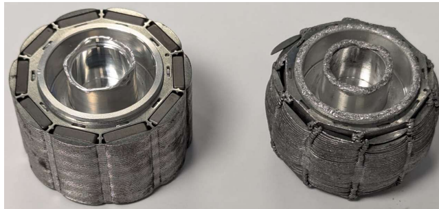
Figure 2. Electric bike motor before and after HPMS processing
