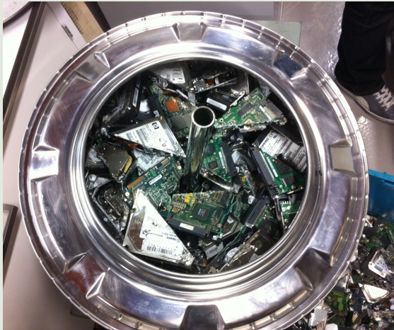
HDDs loaded into porous drum
