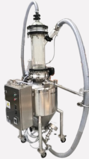
Mobile PTS system for moving powder between processes
